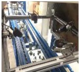
Vision Camera for Thrust washer - Pokayoke
